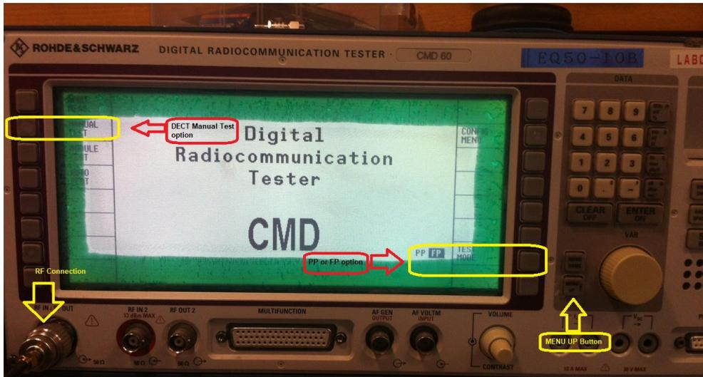
Connect the DUT on the RF Connection (e.g. ANTENNA of DUT to RF IN/RF OUT Terminal)
